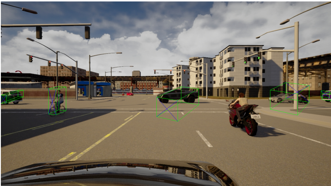
Figure 10.4: Bounding box detection performed poorly. Note, that YOLOv3 missed the motorcycle, thus it is not predicted
