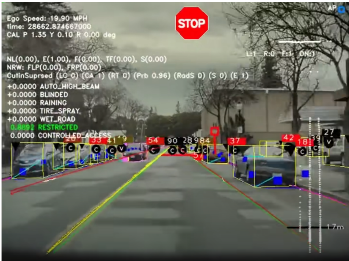
Figure 4.1: A screenshot from a clip that shows Tesla Autopilot's perception output https://www.youtube.com/watch?v=fKXztwtXaGo
