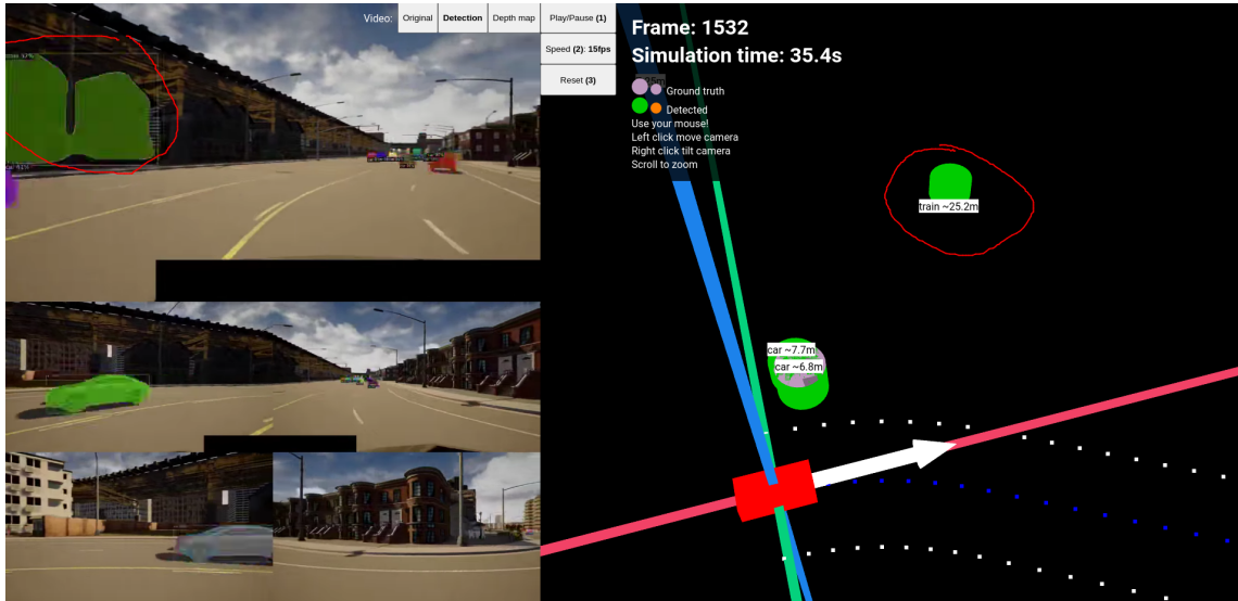
Figure 8.2: False positive detection where a building is detected as a train
